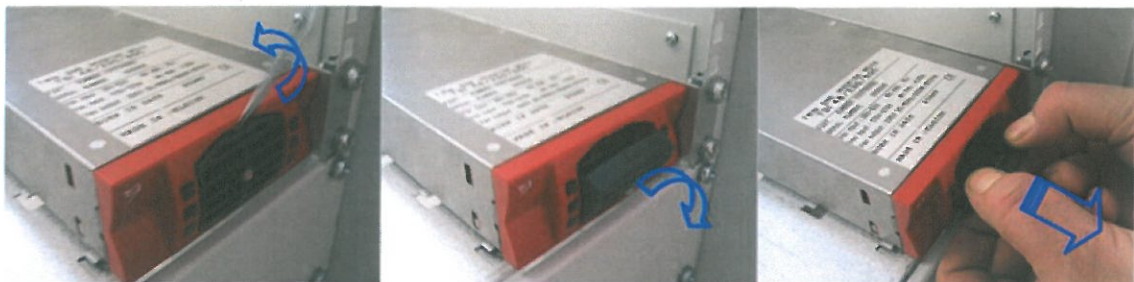
(1) Use screwdriver to release the latch
